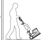
In order for easy transportation, it is recommended to tip the machine as shown in fig.
