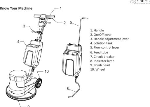
Place the solution tank's bottom tab on the bottom tank holder and press till it sits firmly. Loosen the knob (a) of the top tank holder (b) and move downwards till it gets fixed on the top tab of the solution tank. Adjust the height of the tank placement for ease of operation Tighten the knob to firmly secure its position. Conne the feed tube to the hose connector firmly to prevent any leakage of solution. The machine is ready for use.
