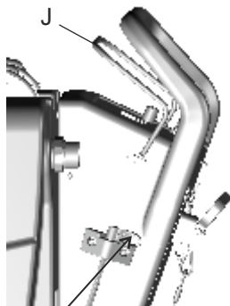
Lever to adjust flow of water
