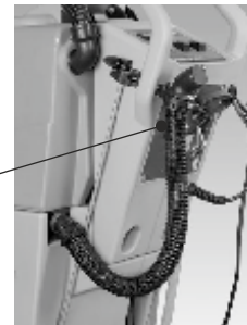
Remove the Hose from this clamp to drain the water
